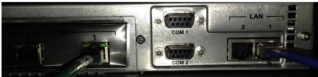
Figure 2. DMG2000 Rear Panel
